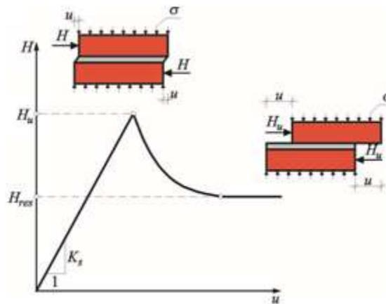
Figure 9: Shear characteristic of interface elements (Stage III)
