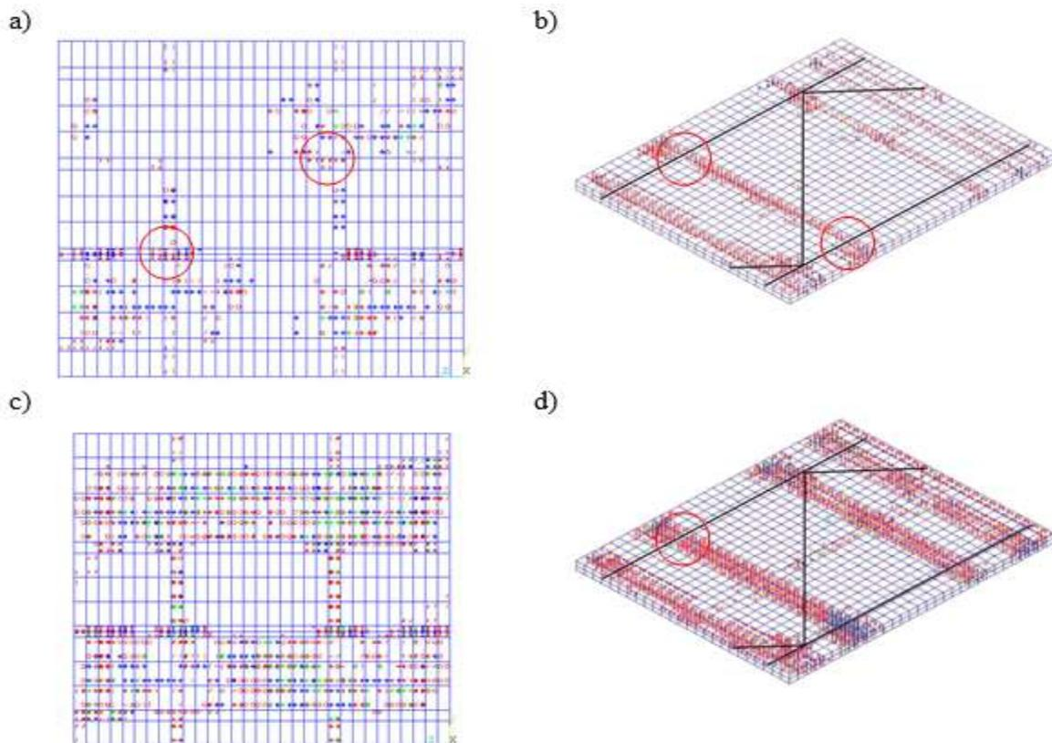
Figure 15: Cracking patterns of reinforced with smooth bars model HC-ZKII-15 series
