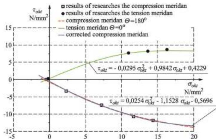
Figure 5: Corrected tensile and compressive meridians of mortar
