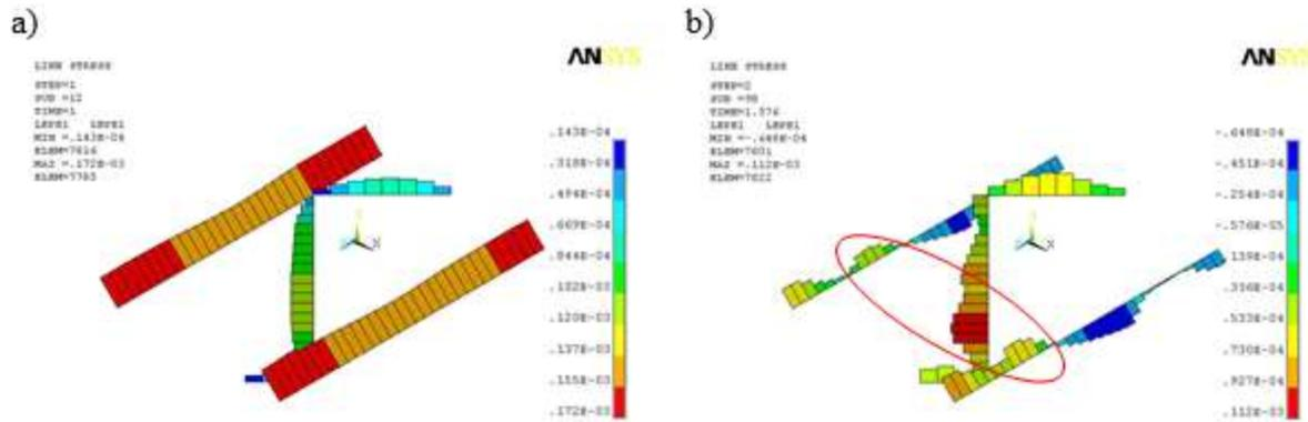
Figure 16: Strains of the truss type reinforcement in successive phases of the load HC-ZKII-15 series: a) initial compression  $H = 0$  kN, b) the destruction of model  $H_{u,cal} = 576$  kN
