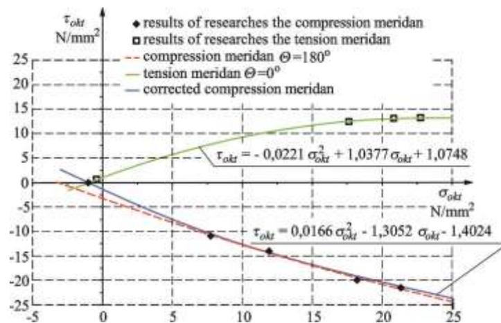
Figure 6: Corrected tensile and compressive meridians of brick
