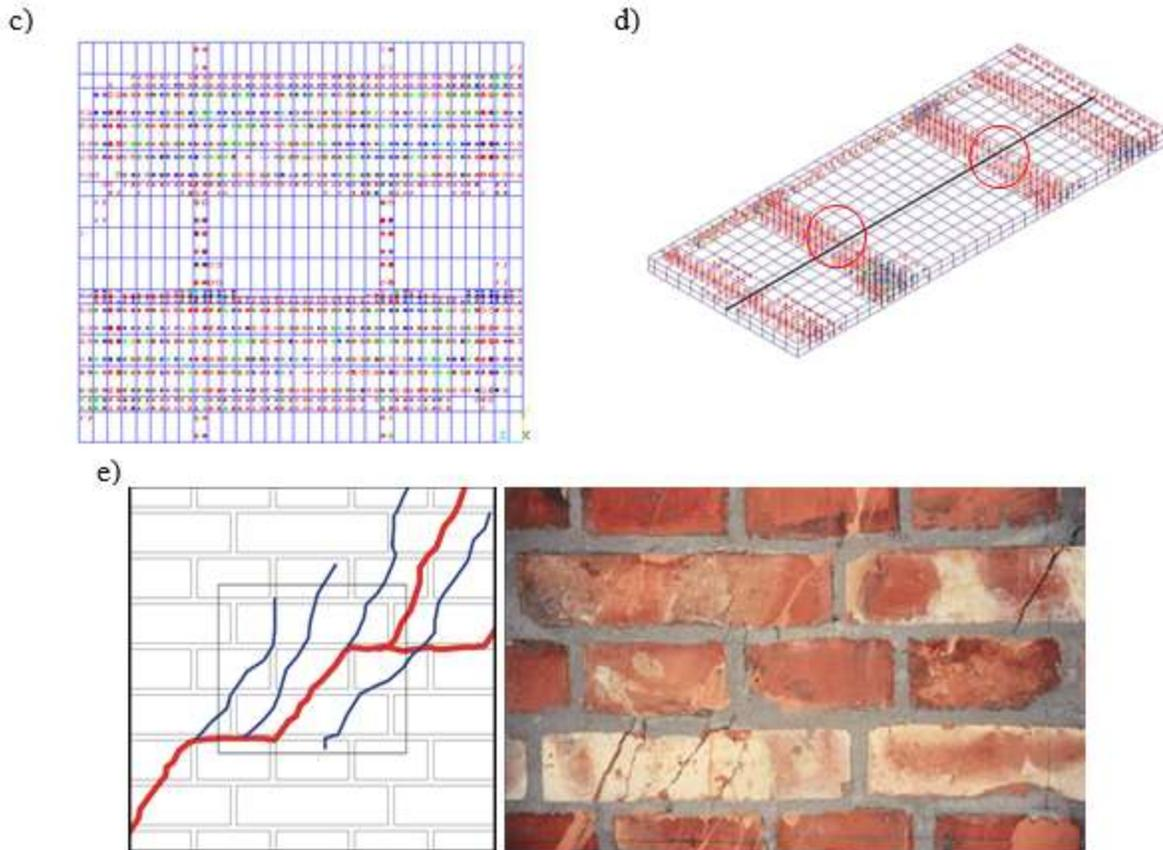
Figure 13: Cracking patterns of reinforced with smooth bars model HC-ZPII-15 series
