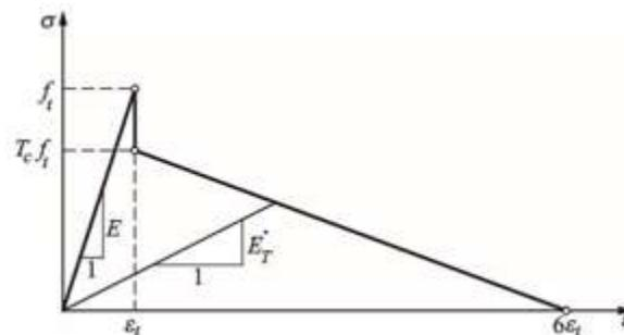
Figure 7: Smearred band of cracks  $\sigma - \epsilon$  relationships
