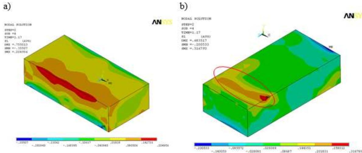
Figure 22: Principal stress  $\sigma_1$  in brick of wall reinforced with truss type reinforcement (HC-ZKII-15)  $H_{cr,cal} = 170$  kN: a) brick over reinforced bed joint, b) brick over reinforced bed joint
