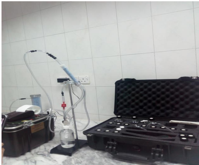
Figure 4: Radon measurement in ground water samples in the Laboratory
