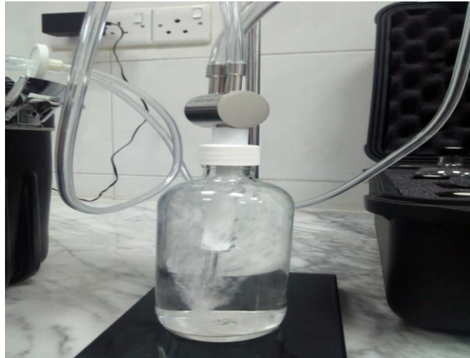
Figure 5: Aeration stage during radon measurement
