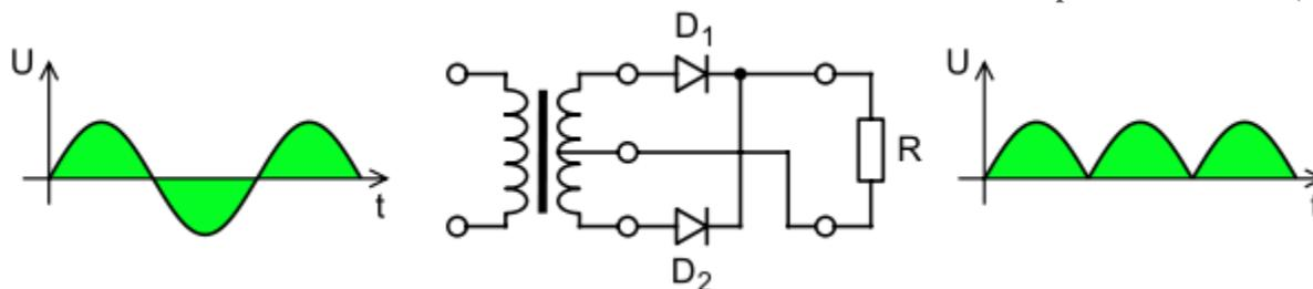
**Figure 4:** Full-wave rectifier using a center tap transformer and 2 diodes.
