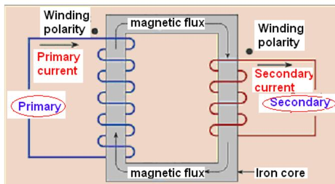
Figure 5: Transformer work
