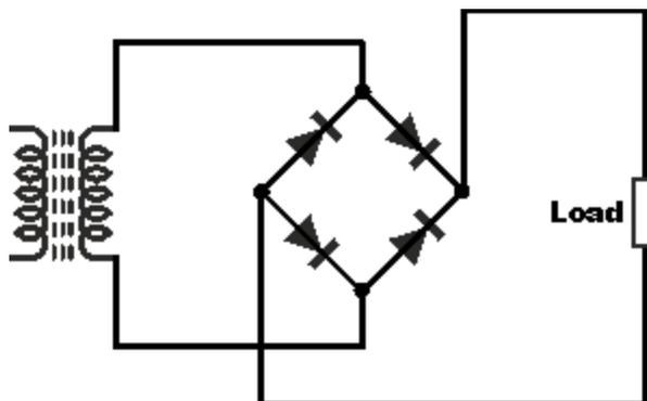
Figure 3: Full-wave rectifier using 4 diodes.
