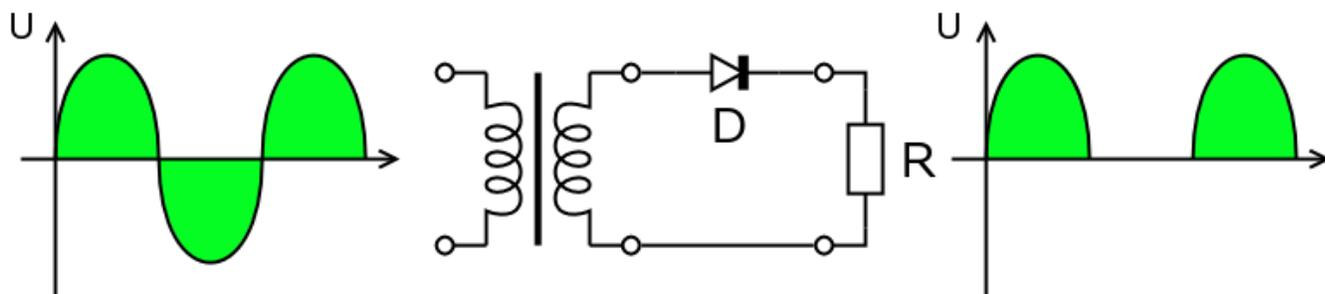
Figure 2: Half-wave rectifier
