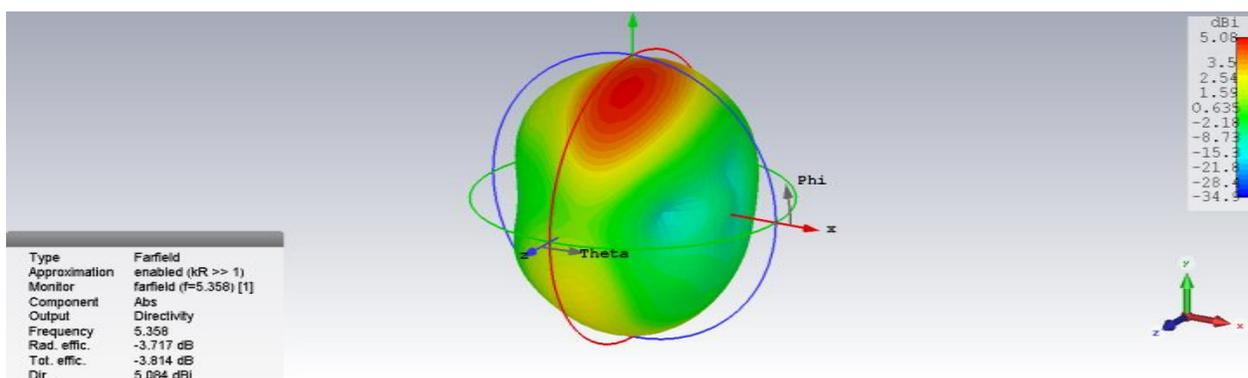
Figure 7: Directivity of MIMO antenna at 5.3 GHz
