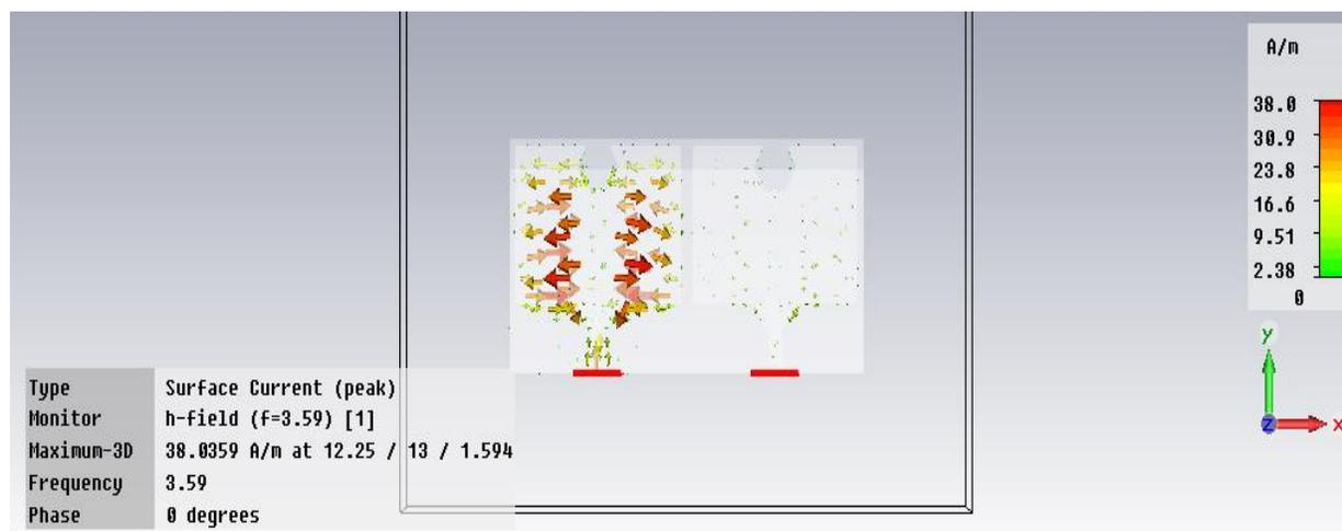
Figure 9: Surface current distributions at 3.59 GHz port 1
