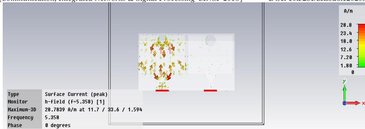
Figure 10: Surface current distributions at 5.35 GHz port 1
