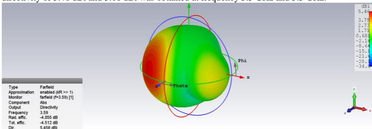
Figure 6: Directivity of MIMO antenna at 3.5 GHz
