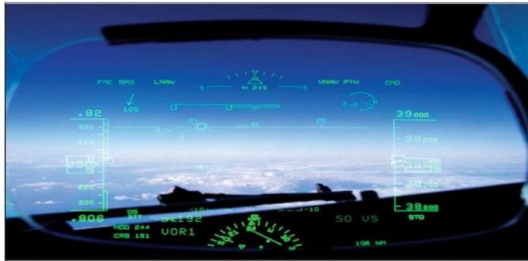
Figure 2: Typical Head Mounted Display of an aircraft showing data like Speed, Altitude, Horizontal line and more
